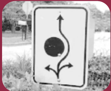
Some neighborhood traffic circles allow left-turning vehicles to pass to the left of the central island.
