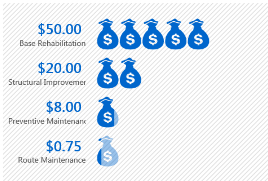
Figure IV-26: Cost Comparison of Pavement Repair Strategies
